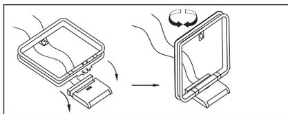
6. Connect the supplied FM antenna to the **FM (75-ohm) Connection 1**. The FM antenna may be an
